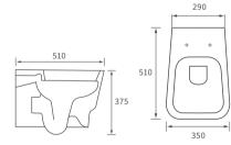
WALL HUNG PAN Coupling to soil stack: Straight out and straight down Distance from soil pipe spigot to wall: 85mm For use with concealed cistern
